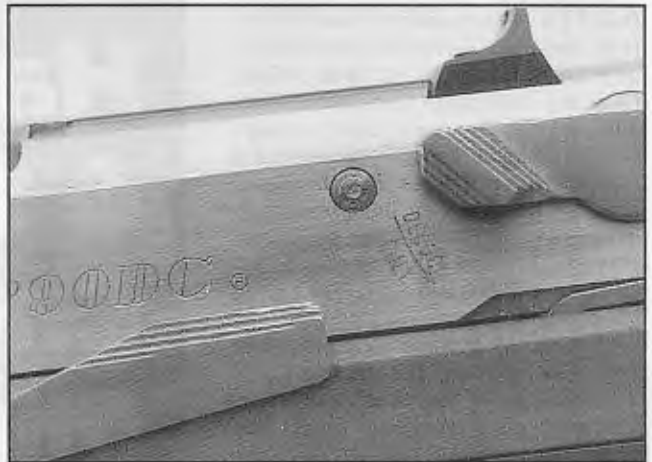
The KP90DC's slide stop lever (left) has taken on an abbreviated form. The ambidextrous, spring-loaded, hammer-drop lever is slide-mounted and will drop the hammer without initiating a manual safety.
